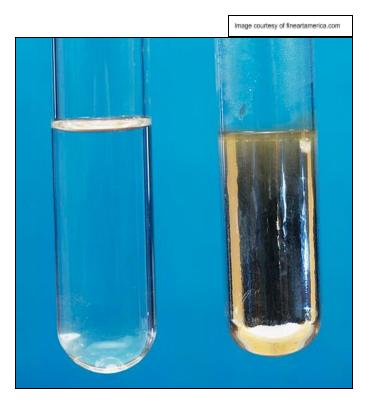
**Fehling's solution** is another way of testing for aldehydes. It is added to the solution being tested and heated. A **brick red precipitate** will form if an aldehyde is present and if not, the solution **remains blue** and there is no observed change.
